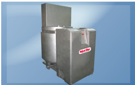
Rühr-Emulsionstank RMT-1000 COOL
